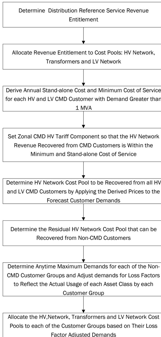
Figure 2 - Distribution Cost of Supply Flow Chart
